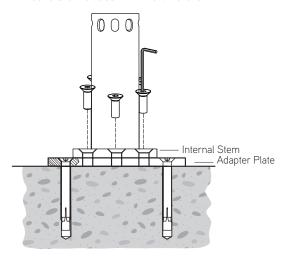
Insert (4) expansion bolts into countersunk holes and tighten using a 6mm hexagon wrench.
