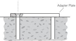
Concrete should be at least 6"thick (8" thick concrete required for rooftop applications)
