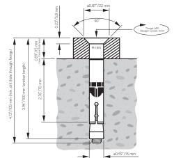
Make sure all adapter plate holes align with drilled holes in concrete.
