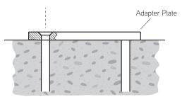
Concrete should be at least 6"thick (8" thick concrete required for rooftop applications)
