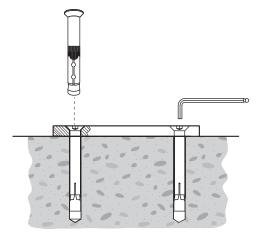
Align internal stem holes with adapter plate holes. Insert (4) stem bolts and tighten using a hexagon wrench to secure. Note: Internal stem and stem bolts are included with the umbrella.
