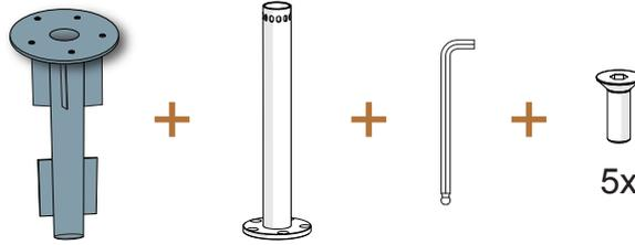
**1** To achieve the exact desired position of the JCP201/301, it is imperative that the installation fitting and internal stem be aligned correctly. One of the 5 internal stem holes must face direction of umbrella.
