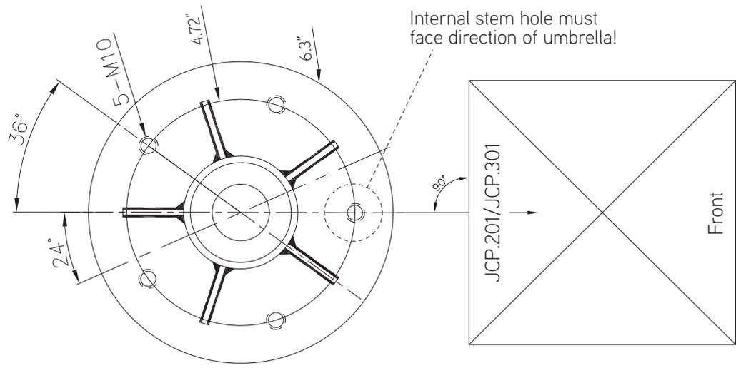
**2** Dig an approximate 90cm/3ft. deep by 60cm/ 2ft. wide hole. Insert in-ground fitting and pour mixed concrete into hole around fitting. Make sure in-ground plate is level.
