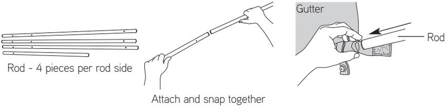
2. Using a two-person team, attach gutter end to ribs, starting closest to mast first. Secure gutter to rib ends by pulling out the self-locking canopy fastener on end of gutter and attach fastener to male button located on rib, and release.
