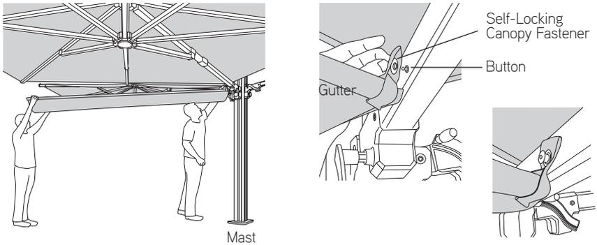
3. Attach other end of gutter (velcro end) to button located near both rib ends. Repeat step 2-3 as necessary (depending on number of gutters installing).
