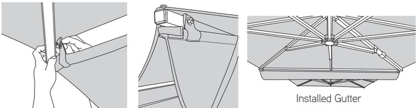
**IMPORTANT:** Remove gutters prior to using tilt function or opening and closing.
