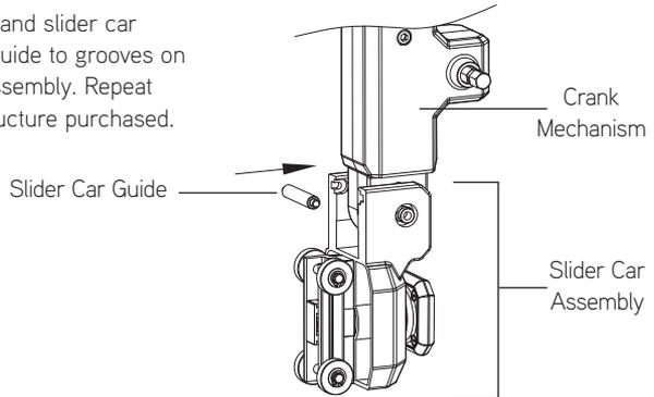
3. From bottom of mast, insert slider car wheels onto 1 side of mast. Repeat for each canopy structure purchased. NOTE: For P2 set up, insert slide cars onto 2 sides of mast you wish to configure.
